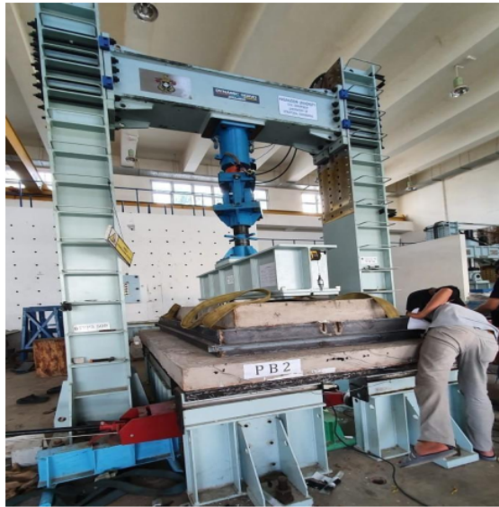
Figure 10. Hollow Plate Loading Pattern (PB-2)
