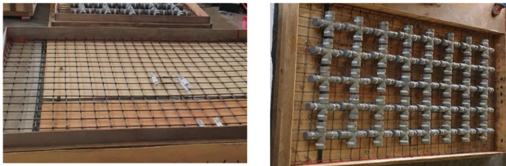
Figure 7. Solid Plate (PP-1) and Hollow Plate (PB-2)
